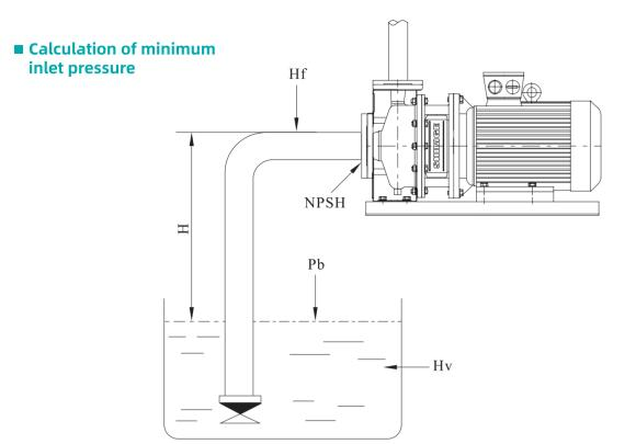
Inlet pressure: In order to ensure that the water pump is in the best operating state, and control the noise at the minimum level, the inlet pressure must be correctly calculated and set. If the pressure in the pump is lower than the vaporization pressure of the conveyed medium, cavitation will occur to the water pump, and in order to ensure a minimum pressure at the inlet of pump, the maximum suction height (m) can be calculated by the following formula:
