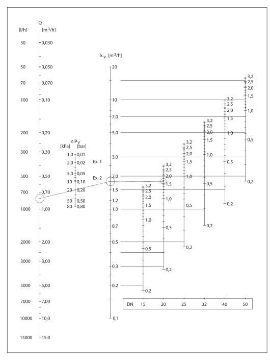
A straight line connecting the bars of flow, differential pressure and k<sub>V</sub> value shows the relationship between these three variables.
