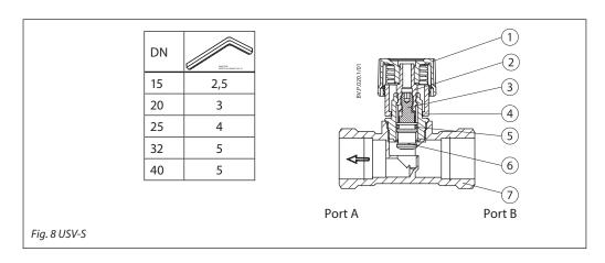
USV-S incorporates a double cone (3.6) able to give maximum stroke limitation, thus achieving flow limitation. It also incorporates shut off function.
